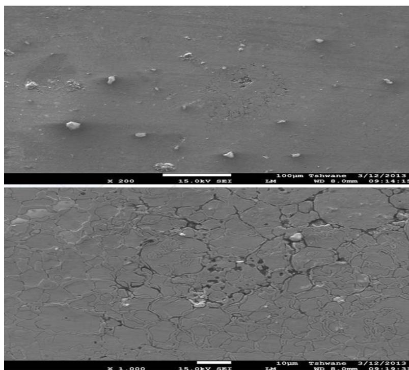
**Figure 5.** Representation of SEM image of corroded sample in simulated mine water at different magnification.
