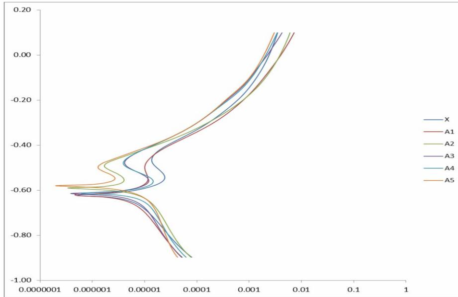
**Figure 4.** Polarization curves of PM 2205 duplex stainless steel composite in simulated Mine water
